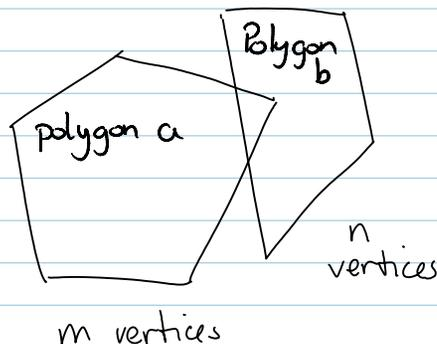
Recall: Collision checking approach of section 4.3 is  $O(mn)$ .
