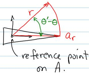
The greatest displacement any point  $a \in A$  can experience is bounded by  $r|\theta' - \theta|$
