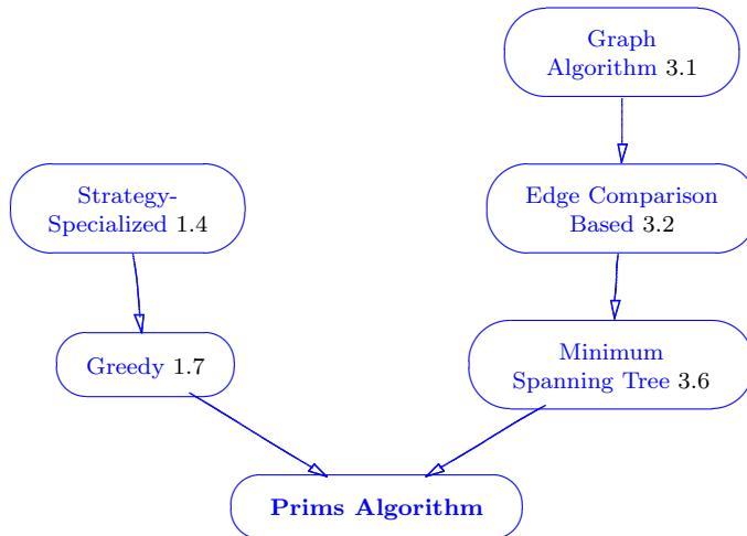
**Refinement of:** Greedy (§1.7) Minimum Spanning Tree (§3.6). Prim's algorithm is a greedy algorithm for solving the Minimum spanning tree problem. It is closely related to Dijkstra's (§3.16) single source shortest path algorithm.
