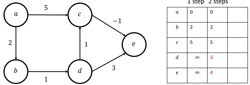
Loop through all 1-step nodes and see if you can reach other nodes in 1 step at lower cost
