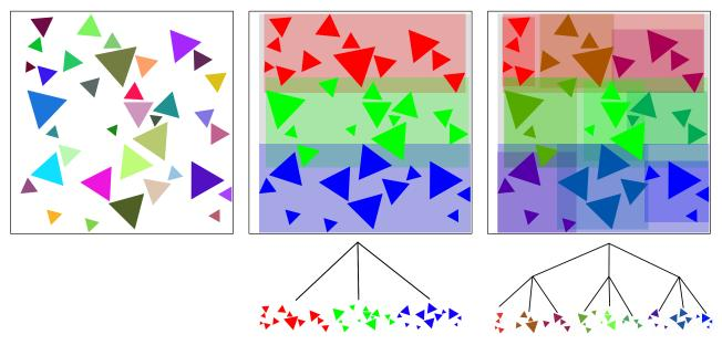
The individual geometric shapes are only stored in the leaf nodes. Every shape is only stored in one leaf node! Every node in the BVH stores the *bounding box* of all of the data stored in that subtree of the BVH. Here's another small example dataset using disks:
